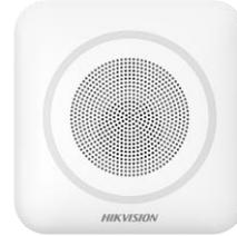
The wireless internal sounder DS-PS1-II-WB, supporting 433MHz two-way communication via Cam-X protocol, multiple alarm sounds, strobe light indication, is used for instant alerting when alarm triggered. Meanwhile, it supports two-way audio function for ARCs to do the alarm verification, which can help the users to know what is the real situation on-site immediately.
